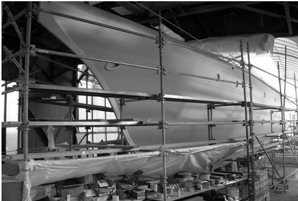
Figure 2 - The hull ready for painting.
