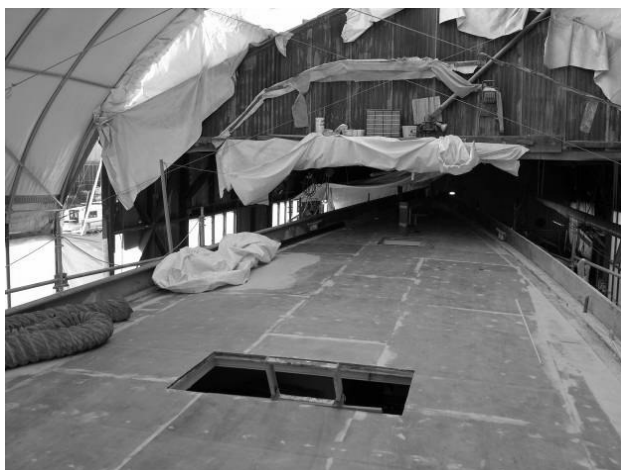
Figure 4 - Deck: two layers of plywood prior to teak.
