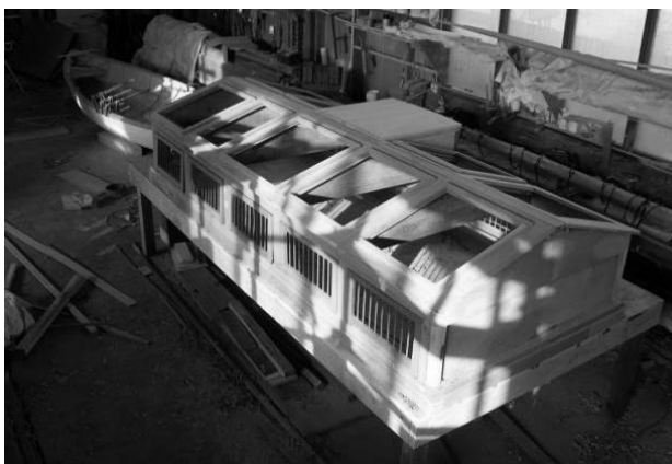
Figure 6- Replication of the engine room skylight showing the grates protecting the side lights.
