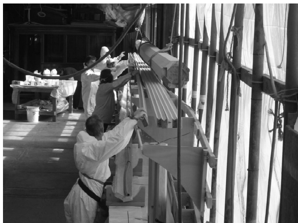
Figure 11 - 65-foot staves are glued into a hollow mast.
