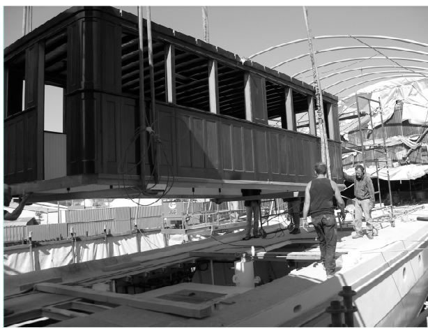
Figure 5 - After cabin being reset on the deck.
